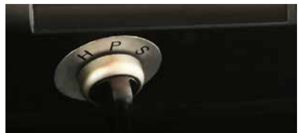
Drive mode selector (H-P-S) to easily personalise the acceleration and the auto-braking effect for each operator's preference
