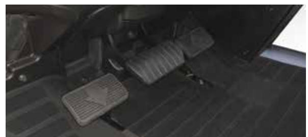
Double accelerator pedal layout
