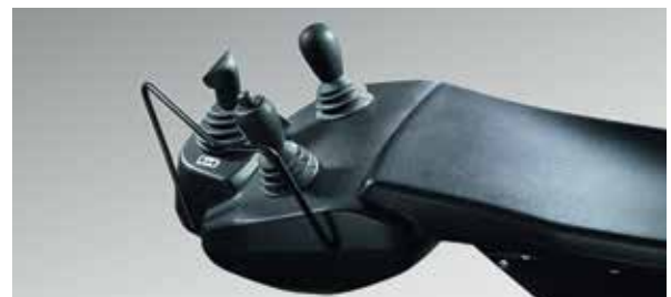
Direction change by lever located at armrest or steering column, also possible with D2 drive pedal
